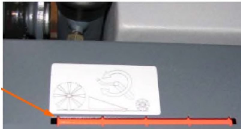
Front edge of pointer plate flush to 1st notch of the mark
